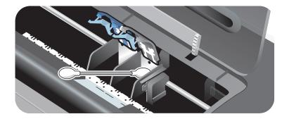
3 Carefully clean the electrical contacts on the print cartridge with a soft, dry, lint-free cloth.
